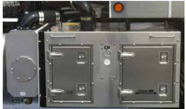
Mounts to truck frame and accommodates right angle gear box or hydraulic drive adapter. (Shown with moisture trap option.)
