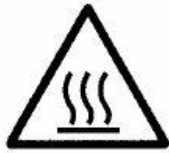
Danger of high temperature
