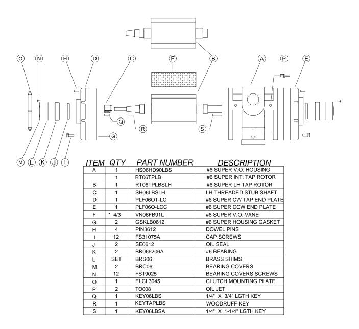
NOTE: PUMP SERIAL NUMBERS PRECEDING #38231 REQUIRE FOUR VANES PER PUMP
