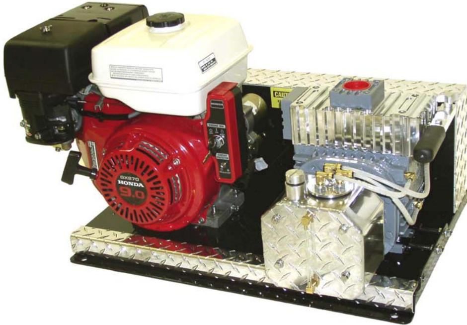
Conde PowerPak gasoline powered vacuum pump units are compact and available with either Conde vacuum/pressure or vacuum only pumps. Electric or pull start Honda engines can be specified. Standard with v-belt drive with beautiful diamond plate belt guard and trim. Conde PowerPak units are ready to quickly install on your system for your vacuum needs. Quality, reliability, and ease of operation!
